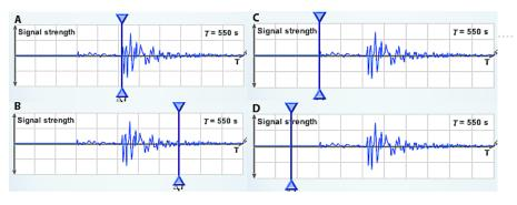
2. Which of the following has the two vertical probes in the proper positions to find the correct value for  $\Delta T$ ?
